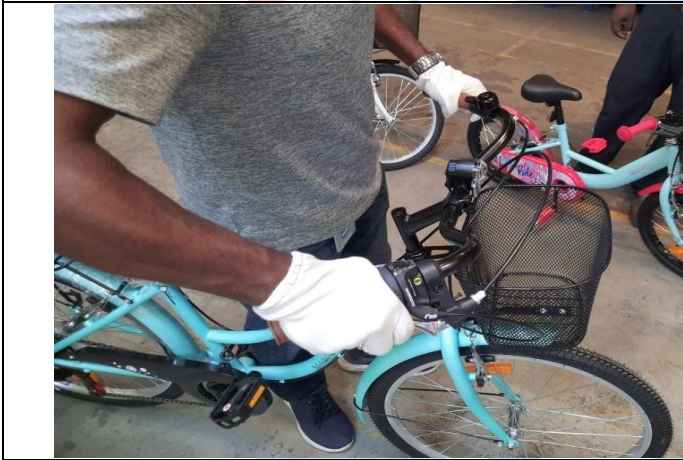
Fork alignment Check
