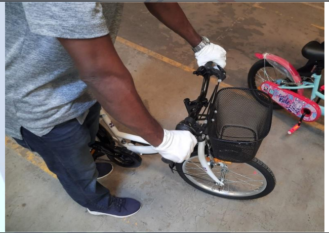
Fork alignment Check
