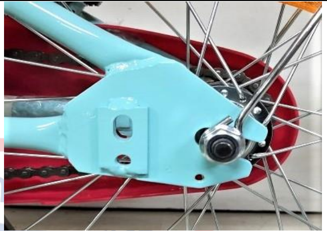
Welded Joint Check
