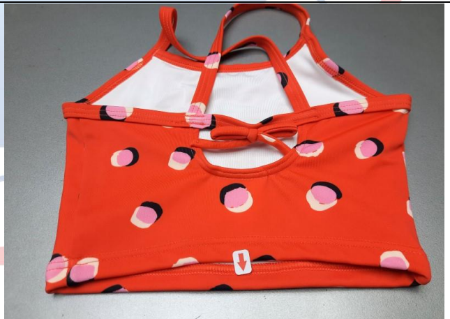
Hiking at back bottom seam - Ma
