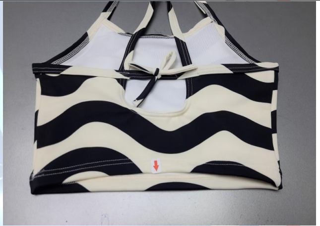
Hiking at back bottom seam - Ma
