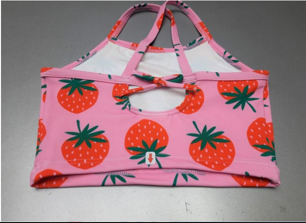
Hiking at back bottom seam - Ma
