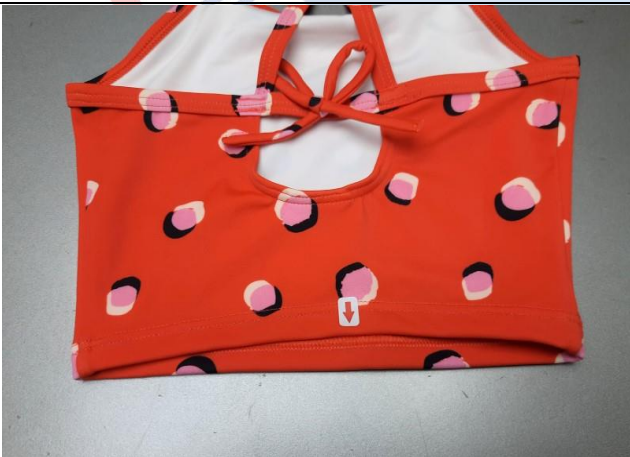
Hiking at back bottom seam - Ma
