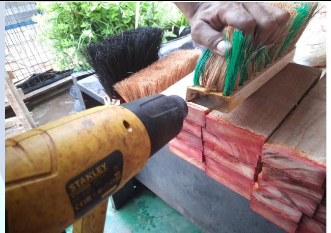
Coat Sodium Borate applied & Heating
